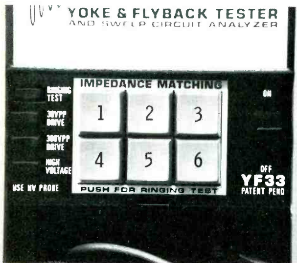
Fig. 3 Six "impedance matching" pushbutton switches select the value of internal capacitance giving the most cycles of ringing. (The numbers are not on the RINGER; we added them to the picture for identification.)
