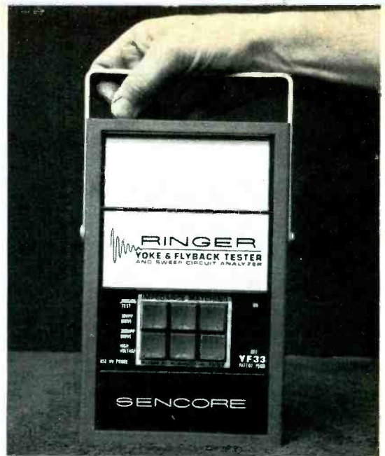
Fig. 10 The meter is protected by a sliding lid, and the power cable and test leads are behind the compartment door at the bottom, when the RINGER is stored or transported.
