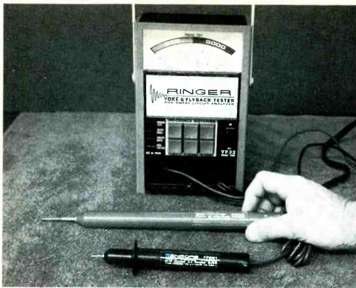
Fig. 9 The black probe (nearest the camera) enables the YF33 to measure up to 10-KV DC, while the larger red slip-on probe extends the range to 50-KV full-scale.
