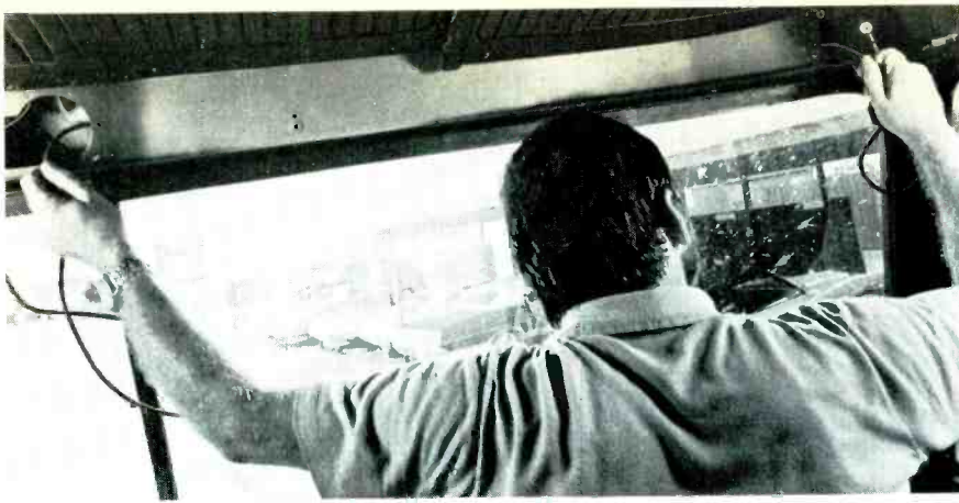
Fig. 5 RG-59U cable is stiff enough that a fish tape should not be necessary to pull the cable through the tunnel over the windshield. Don't forget the grommet for the outside hole.
